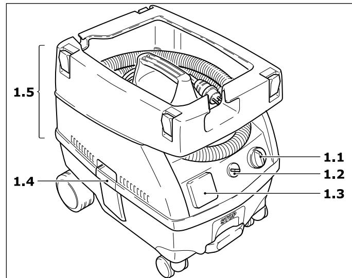
**WARNING** Before turning the switch to the "Auto" position, make sure that the tool connected to the tool plug socket is switched off. When you turn the switch to "Auto" the dust extractor will not come on until you turn on the tool connected to the tool plug socket. When you turn off the tool, the dust extractor will automatically switch off. When you turn the tool back on, the dust extractor will automatically start.
